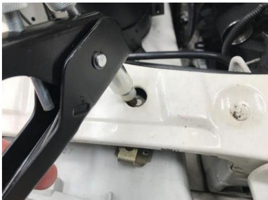
Drill the hole out to 7mm
