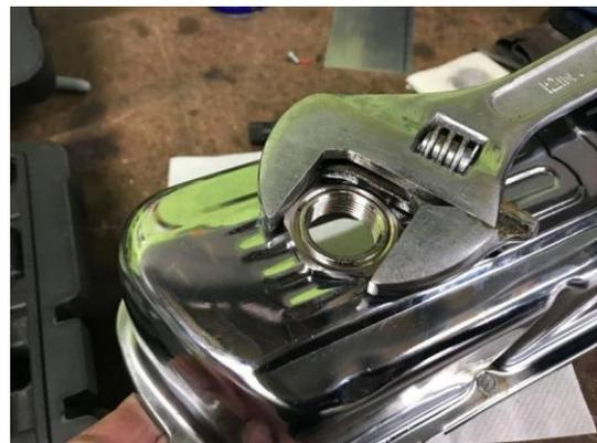
Screw in the cap and reinstall rocker cover back on the motor. I put some water in the rocker cover to check for leaks....found none.
